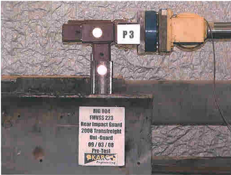
Figure 11. Pre-Test, Location P3
